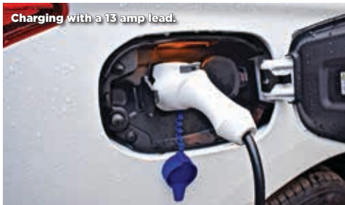
Charging with a 13 amp lead.
